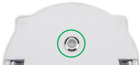
There is a waterproof triple color LED on DLOS8 enclosure, the meaning of the LED is:
