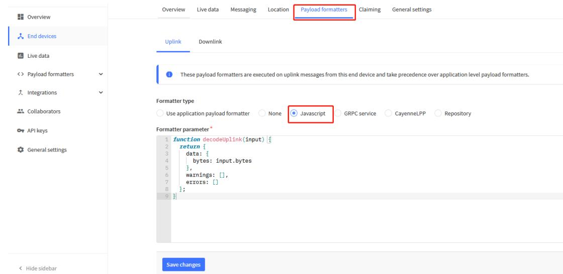
The screenshot shows the TTN V3 web interface with the 'Payload formatters' tab selected. Under 'Formatter type', 'Javascript' is chosen. The code editor contains the following Javascript function:
