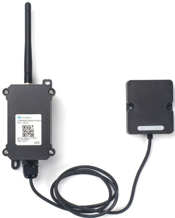
The Dragino LMDS200 is a LoRaWAN Microwave distance sensor. It uses [24Ghz Microwave](#) to detect the distance between sensor and different objects. Compare vs ultrasonic or Lidar measurement method, Microwave Radar is [more reliable for condensation / dusty environment](#). It can sense correct distance even there is water or thick dust on top of the sensor.
