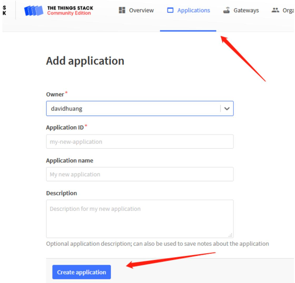
The screenshot shows the 'Add application' page of the TTN V3 interface. At the top, there is a navigation bar with icons for Overview, Applications (which is highlighted with a blue underline), Gateways, and Orgs. A red arrow points from the text above to the 'Applications' tab. The main form has the following fields:
