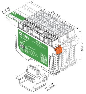
**Installation:** Tilt the module with the rounded corner towards the DIN-rail and then slide and click it onto the connector. As the connector is 22.5 mm wide, the small gap between modules allows for tidy and uncluttered cabling.
