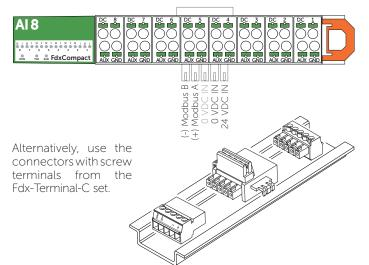
**Modbus address:** The address of the AI-8-C module can be set from 1 to 63 by changing the position of dip-switches 1-6. Each dip-switch represents a binary value, as indicated on the module (ST1...ST32).
