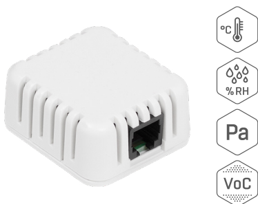
Sensor THPVoc 1W-UNI Temperature range: -30 to +70 °C Humidity range: 0 to 100 % RH Atmospheric range: 30000 to 110000 Pa Air quality range: 0 to 60000 ppb
