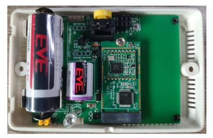
The battery life of LAQ4 is about 7~ 10 months, there are several parameters affect the battery power. Please see consumption report from here for the detail explain: http://www.dragino.com/downloads/index.php?dir=LoRa\_End\_Node/Battery\_Analyze/
