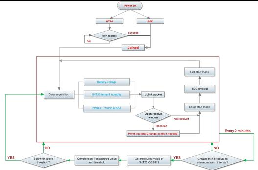
User can use **AT+CO2**, **AT+ATEMP** and **AT+HUM** command to set the alarm low limit or high limit. Device will check CO2, temperature & Humidity every minute, if the temperature lower than low limit or greater than high limit. LAQ4 will send an <u>Alarm packet base on Confirmed Uplink Mode</u> to server.
