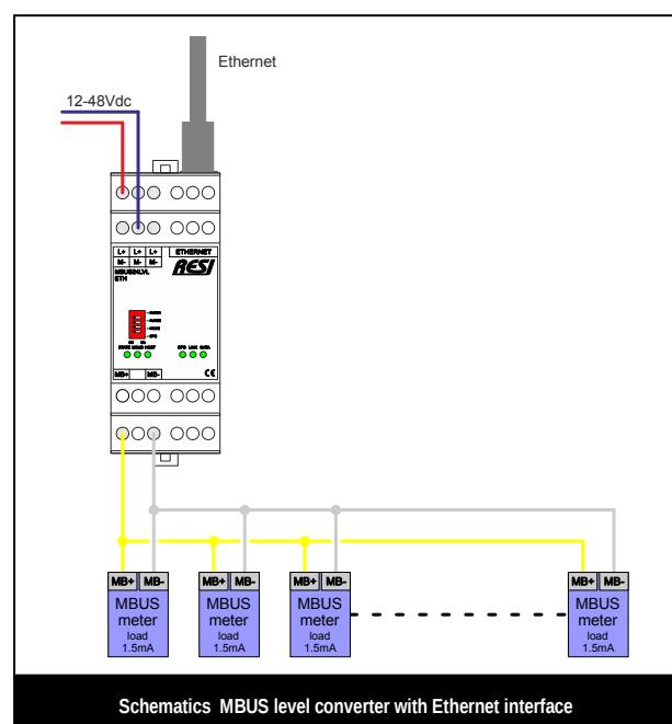
Schematics MBUS level converter with Ethernet interface
