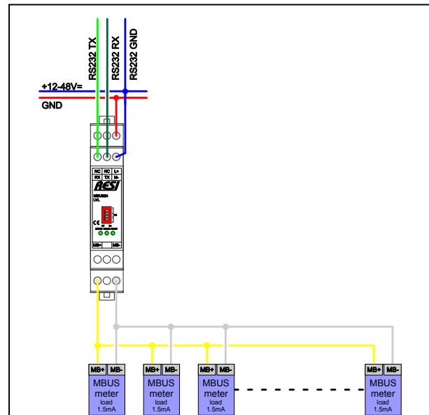
Schematics MBUS level converter with RS232 interface
