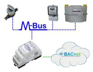
The gateways of the MBUS-GEB product family come with a BACnet software stack which is certified according to PICS (BACnet/IP Annex J). This ensures the compatibility with other BACnet devices.
