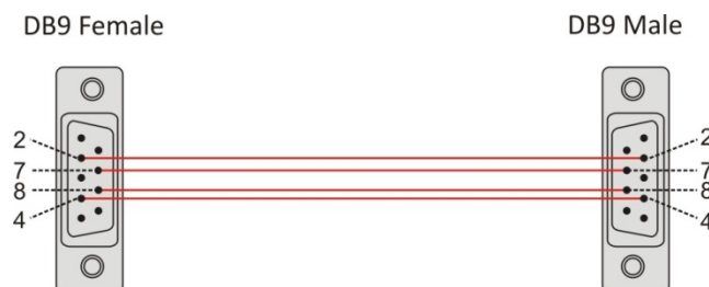
Figure 112 Building an extension cable
