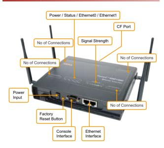
**The Parani-MSP1000** is a Bluetooth Access Point to enable Bluetooth devices to be connected to 10/100Mbps Ethernet network. Parani-MSP1000 supports 7, 14, and 28 Bluetooth connections according to the model, and it supports up to 3Mbps throughput through Bluetooth 2.0+EDR specification. Parani-MSP1000 is a class 1 Bluetooth device that supports 150m using basic dipole antenna and up to 1 km using patch antenna.
