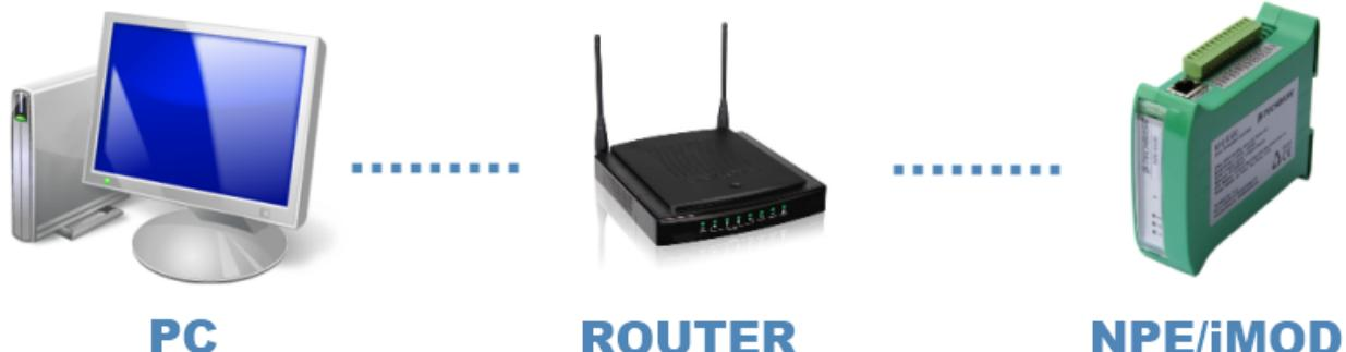
Another method is connecting the device to a local area network (LAN). If a router in the network has the DHCP (Dynamic Host Configuration Protocol) service active, the device IP address will be randomly assigned after start. In order to improve searching for the addresses assigned to devices in the local area network the [SearchNPE](#) application has been created.
