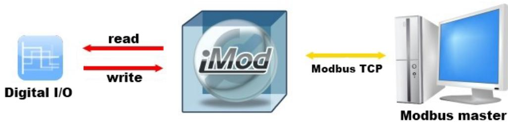
After uploading an appropriate configuration you can gain access to all the input/output resources that the platform is equipped with, using the Modbus protocol.
