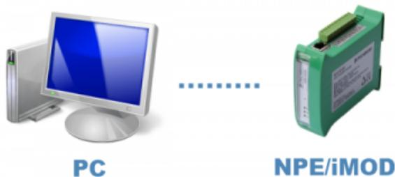
Direct connection between a computer and the device requires additional network interface configuration. The device should be connected directly to a computer with an Ethernet network cable.
