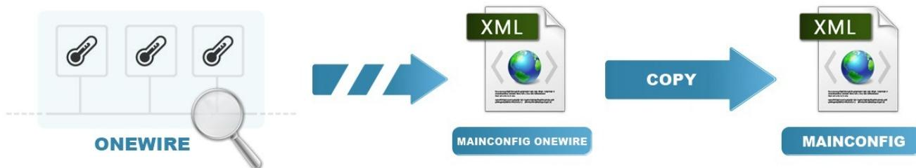
After scanning the one-wire bus you need to copy part of the configuration into the main configuration - the [MainConfig.xml](#) file from the /mnt/mtd/iMod/config directory.
