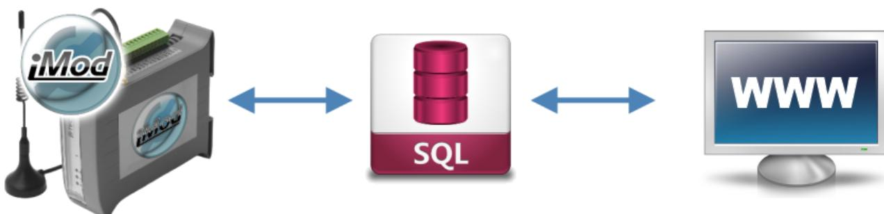
The iMod telemetry module uses a built-in Apache2 web server with PHP and database (SQLite and PSQL) support for sharing data. In order to build a simple web interface you just need to know basics of HTML, PHP and be familiar with database support.
