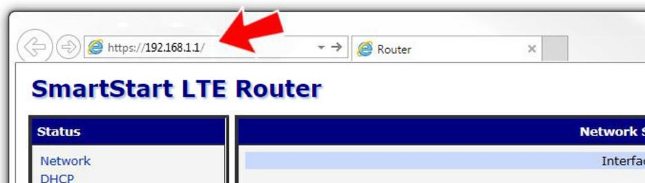
Figure 22: Entering the IP address of the router
