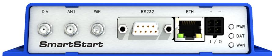
Figure 12: SmartStart front panel
