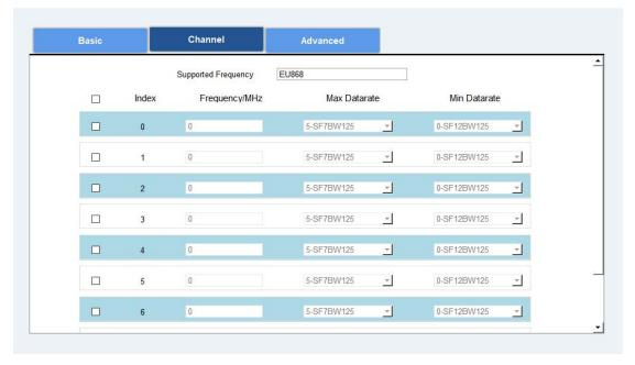
**Note:** Make sure that you have configured the corresponding channel on the gateway. E.g. If you have configured a 923.2 MHz channel on UC1114, then you have to configure a 923.2 MHz channel on gateway as well.
